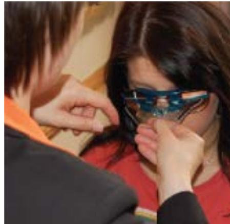
Figure 9: Measurement of face form angle (Courtesy of r+h)
