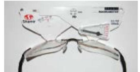
Figure 10: Face form angle gauge Courtesy of Shamir
