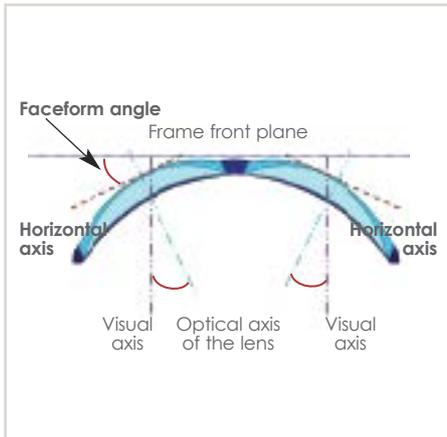
Figure 8: The face form angle (Courtesy of r+h)
